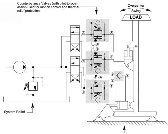
Pilot Check used for position locking on lower cylinder head end:
